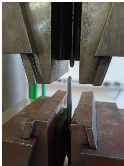
Fig. 7. Destruction of a steel nail: a – formation of the «neck»; b – destruction of the «neck»
