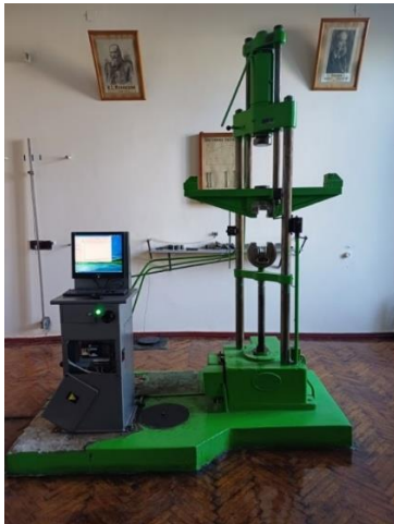
Fig. 3. Measuring unit for testing steel nails
