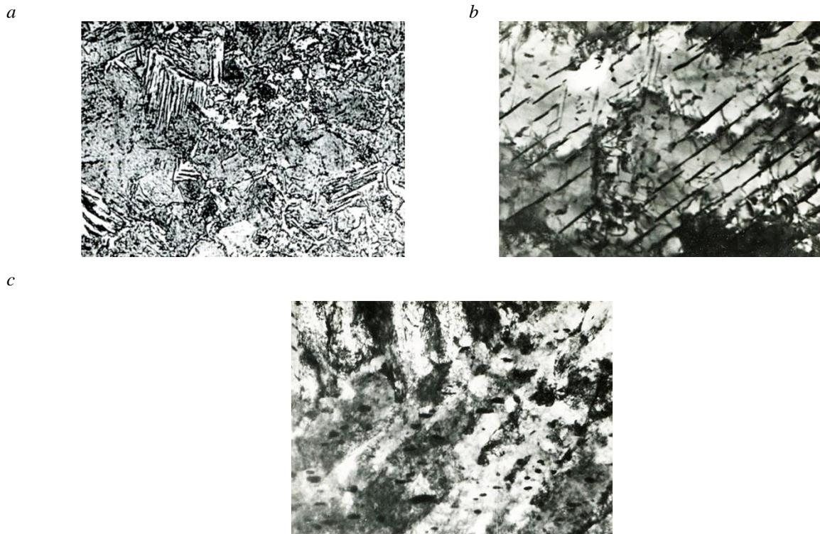
Fig. 3. Structure of the low-carbon steel after isothermal transformation at temperature of 300 °C. Magnification: *a* – 1000; *b, c* – 18000
