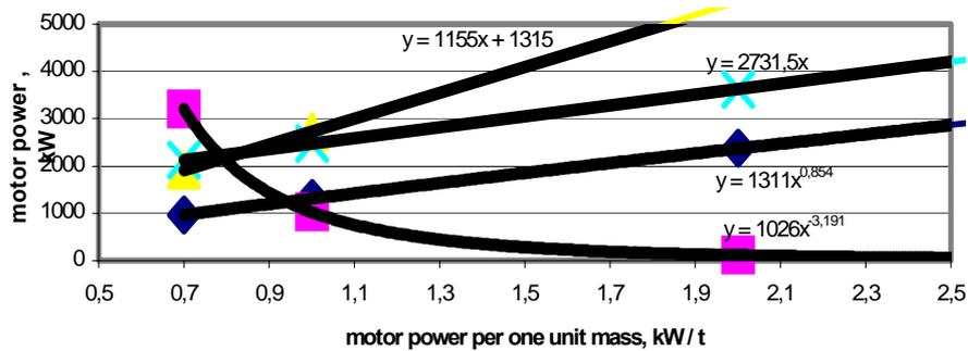
Fig. 4. Optimal motor power depending on motor power per one unit mass
