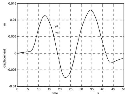
Fig. 16. Lateral displacement of wheelset and car body
