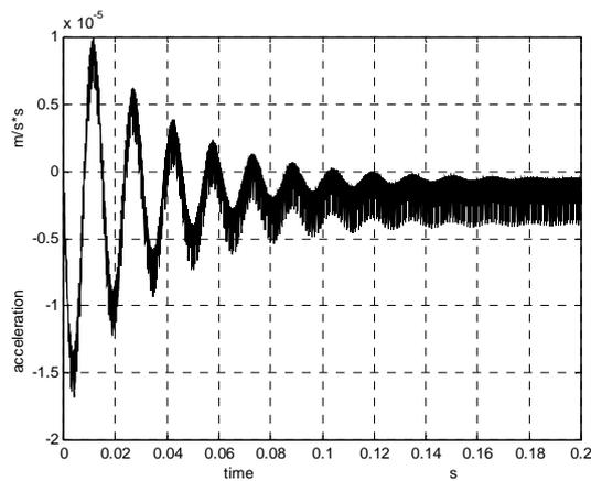
Fig. 7. Lateral oscillations of the car body
