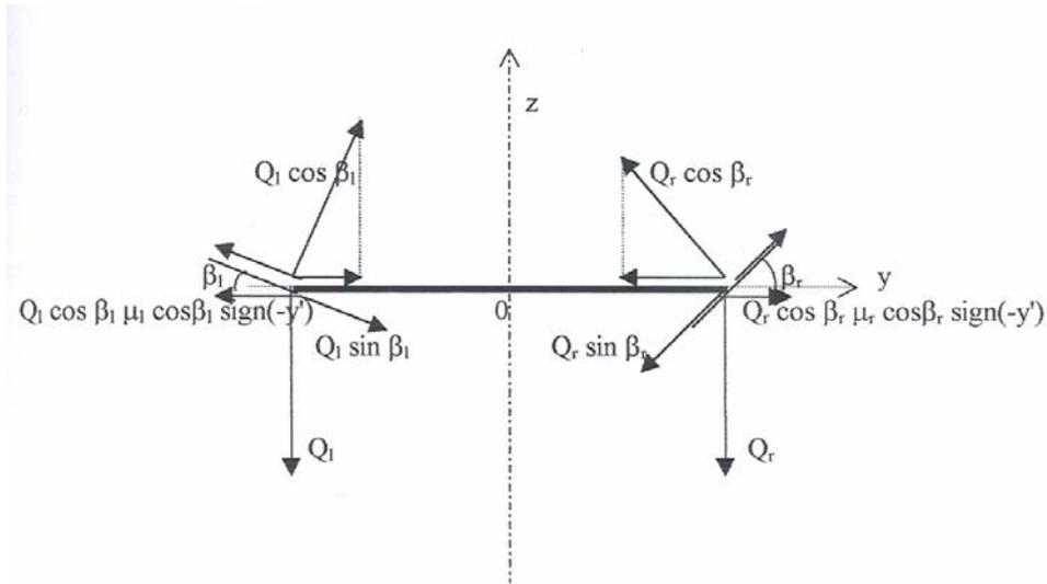
Fig. 3. Lateral forces on the wheel flange
