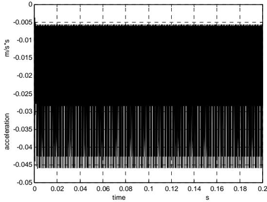
Fig. 6. Lateral oscillations of the wheelset
