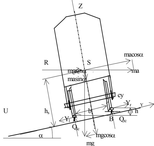
Fig. 11. Scheme of the lateral oscillating system vehicle-rail in the railway line curve
