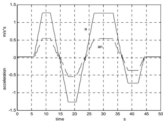
Fig. 14. Total and non-compensated lateral acceleration
